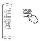
Use the VIDEO ON/OFF button to turn video output to the television (monitor) on and off. It is not necessary to turn video off, but you may notice a slight improvement in audio quality if you turn off the video when playing back SACD discs and CDs without video images.
